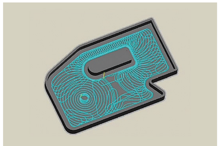
DYNAMIC MILL® MODERATE FORCE HYBRID TOOLPATH Machine and tool capacity utilization up to 75 percent
